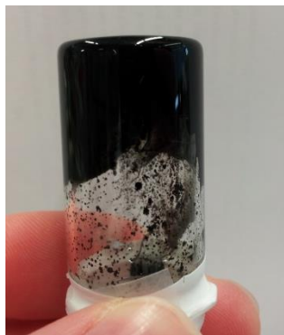
Figure S3. Digital photograph of an unsuccessful functionalization experiment with a polystyrene- block -polybutadiene- block -poly(methyl methacrylate) ( S_{340}B_{340}M_{360} ) triblock terpolymer (CNT1/SBM = 2/1 (w/w) in toluene, overall concentration of c = 30 g/L).
